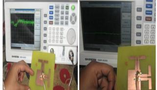
Fig:3 Co-polar and cross-polar levels of the dual printed dipole antenna measured on spectrum analyzer.
