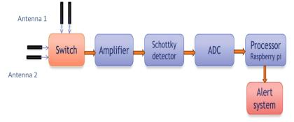
Fig:1. System Block Diagram
